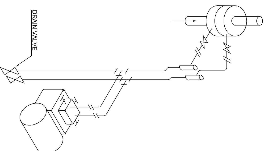
IMPULSE PIPING FOR STEAM FLOW MEASUREMENT (ORIFICE, NOZZLE, VENTURI)
