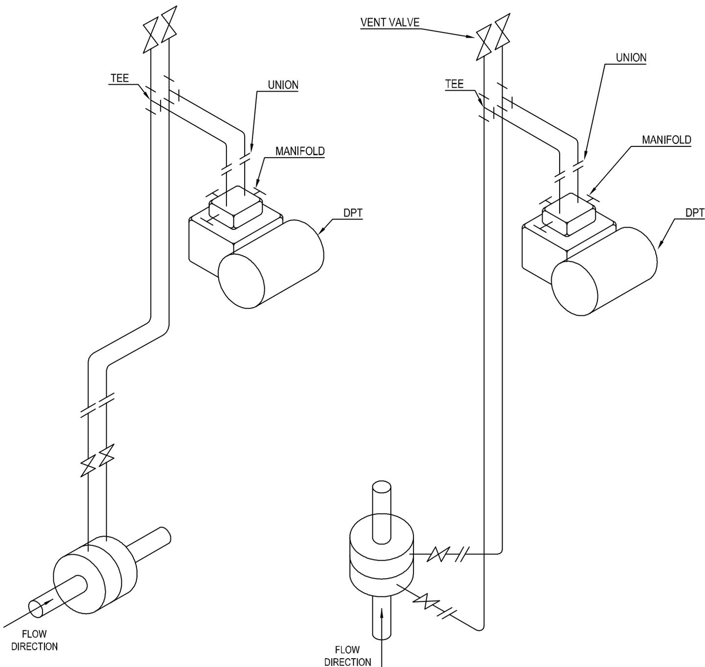
IMPULSE PIPING FOR GAS FLOW MEASUREMENT (ORIFICE, NOZZLE, VENTURI)
