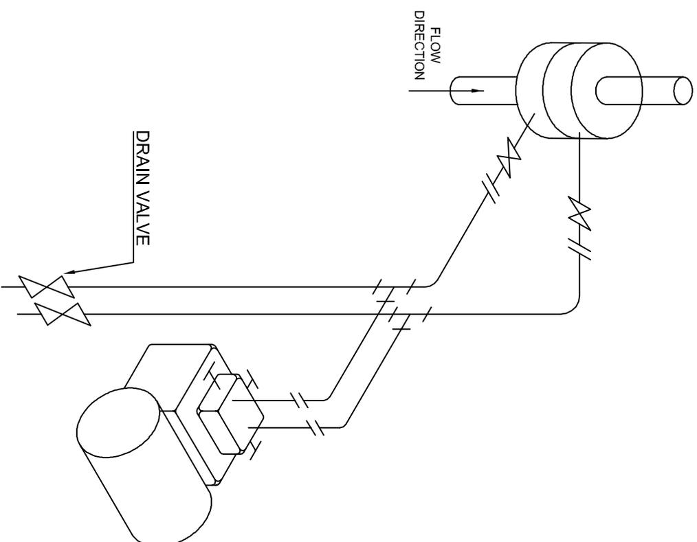
IMPULSE PIPING FOR LIQUID FLOW MEASUREMENT (ORIFICE, NOZZLE, VENTURI)
